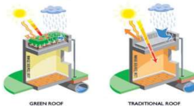
Fig (3) The ability of green roofs to retain rainfall when compared to other types of roofs
